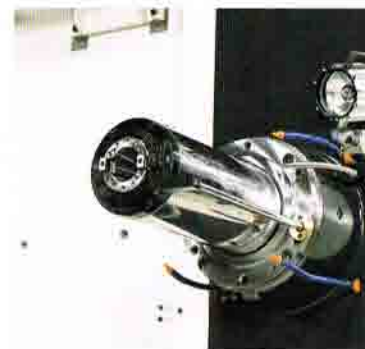
3 Spindle nose coolant (through-tool type) 23 Coolant/air blow unit
