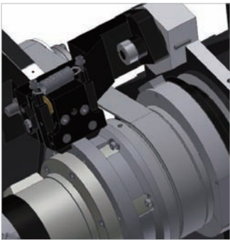
Sub spindle C-axis angle encoder and brake
